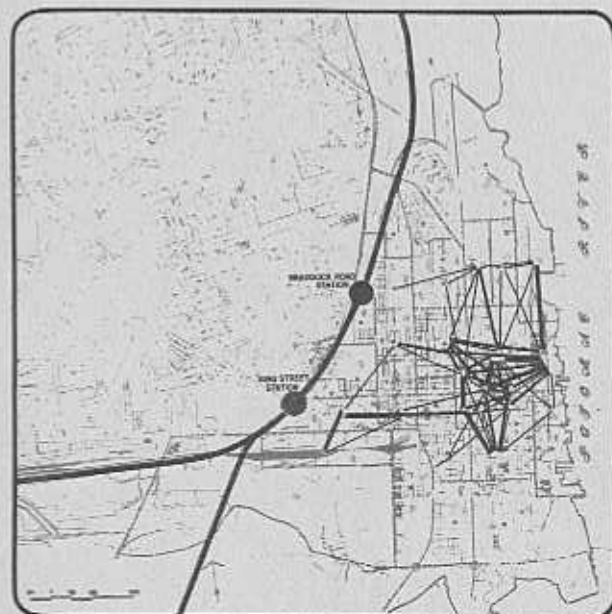
Figure 21 Desire Lines for Daily Downtown Trips (AND COMMERCIAL MODEL, HIGH MODAL SPLIT)
