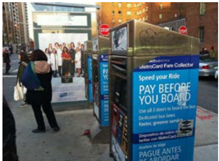
An off-board fare payment system utilized by the New York MTA's Select Bus BRT system. Photo by Flickr user Phil Davis NY. Licensed under Creative Commons
